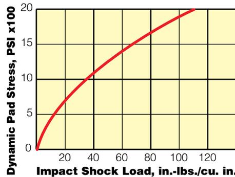
**NOTE:** Large impact shock loads coupled with high impact frequencies can develop considerable heat and therefore shorten pad service life. At impact loads of 11 in. lbs./cu. in. under forging hammer anvils and impact frequencies typical of these operations, decades of service life can be expected.
